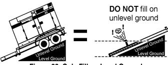
Figure 33. Only Fill on Level Ground
